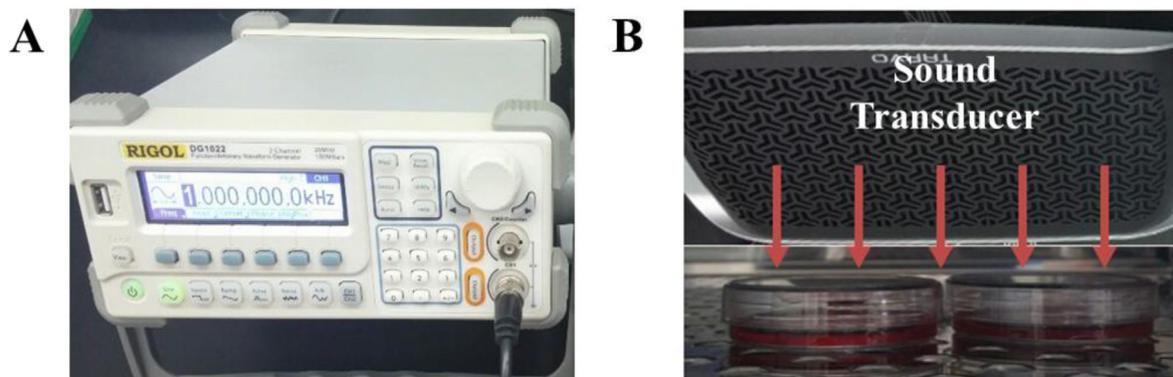
**Fig. 1.** Photo images of the machine used in this experiment. (A) A sound generator installed outside the CO<sub>2</sub> incubator (B) Sound transducer installed inside. The sound generator produced a sound at 1 kHz, 81 dB (0.125 μW/cm<sup>2</sup>). Cells were exposed to sound twice (during 15 min every 12 h) per day for 3 d.
