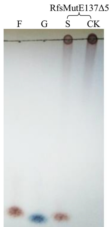
Fig. 5. TLC analysis. Lanes: G, 1.0% (w/v) glucose; F, 1.0% (w/v) fructose; S and CK, inulin with the active and inactivated enzymes, respectively.
