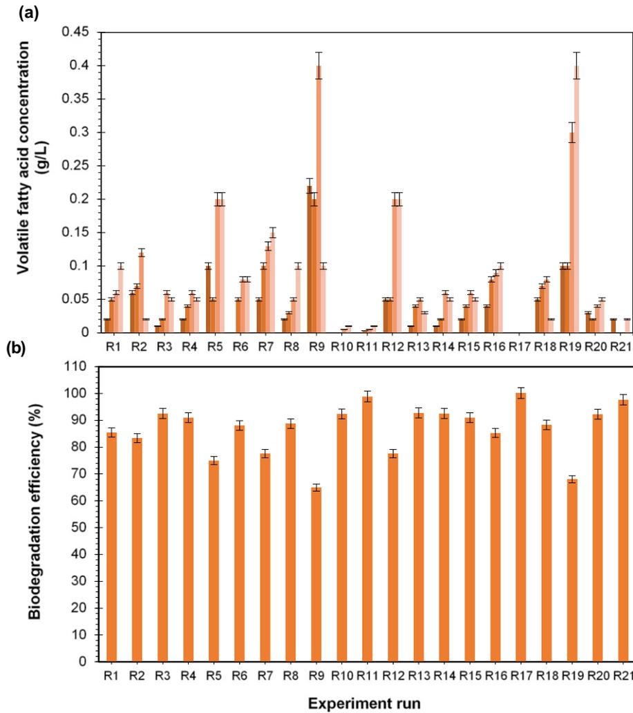
**Fig. 3.** Concentrations of lactic acid, acetic acid, butyric acid and propionic acid in fermentation liquid at the end of incubation (a) and biodegradation efficiency (b) from POME hydrogenic effluent with additions of VFA.
