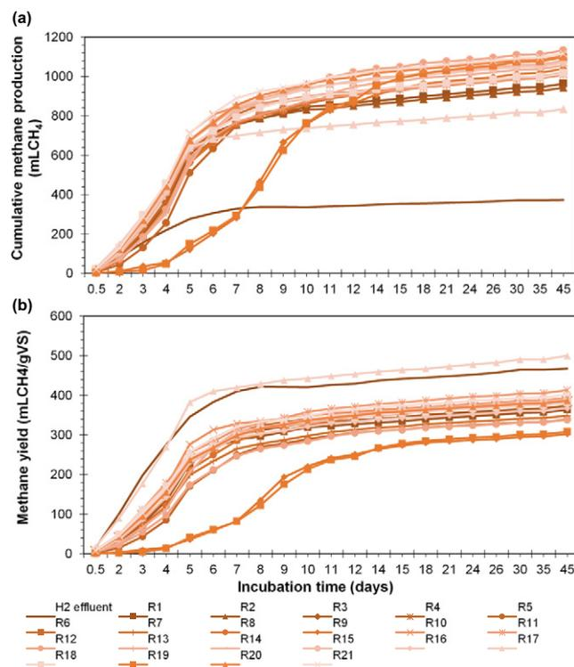
Fig. 2. Cumulative methane production (a) and methane yield (b) from POME hydrogenic effluent with additions of VFA at different concentrations.
