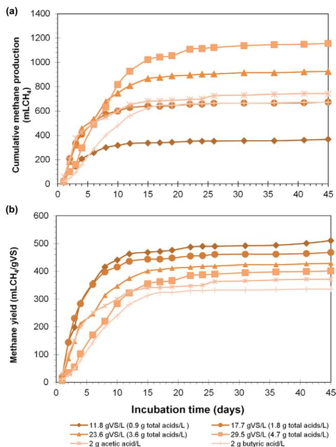
Fig. 1. Cumulative methane production (a) and methane yield (b) from POME hydrogenic effluent.
