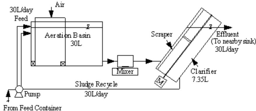
Figure 1. Bench scale CFSTR system.
