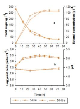
Fig. 6 Fermentation kinetics during batch ethanol production from the sweet sorghum juice supplemented with 8 g  $\Gamma^1$  of DSY in 5-litre and 50-litre bioreactors. (a) total sugar (closed symbol) and ethanol concentration (open symbol), (b) log viable yeast cells (closed symbol) and pH (open symbol).
