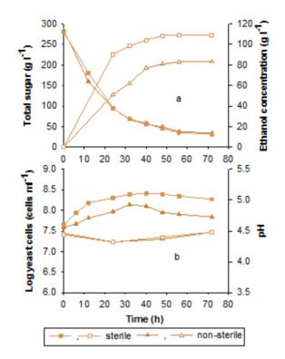
Fig. 4 Fermentation kinetics during batch ethanol production from sterile and non-sterile sweet sorghum juice supplemented with 8 g  $\Gamma^1$  of DSY by *S. cerevisiae* NP01. (a) total sugar (closed symbol) and ethanol concentration (open symbol), (b) log viable yeast cells (closed symbol) and pH (open symbol).
