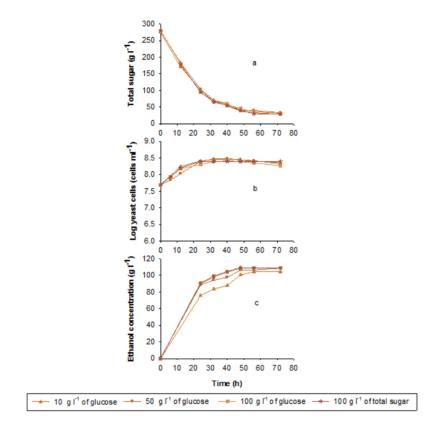
Fig. 3 Fermentation kinetics during batch ethanol production from the sweet sorghum juice supplemented with 8 g  $\Gamma^1$  of DSY by *S. cerevisiae* NP01 grown in different initial sugar concentrations in IP medium. (a) total sugar, (b) log viable yeast cells and (c) ethanol concentration.
