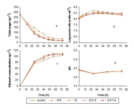
Fig. 1 Fermentation kinetics during batch ethanol production from the sweet sorghum juice containing 280 g  $i^{-1}$  of total sugar under various nitrogen supplements by *S. cerevisiae* NP 01. (a) total sugar, (b) log yeast cells, (c) ethanol concentration and (d) pH.
