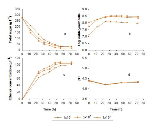
Fig. 2 Fermentation kinetics during batch ethanol production from the sweet sorghum juice supplemented with 8 g  $I^{-1}$  of DSY under different initial yeast cell concentrations of *S. cerevisiae* NP 01. (a) total sugar, (b) log viable yeast cells, (c) ethanol concentration and (d) pH.
