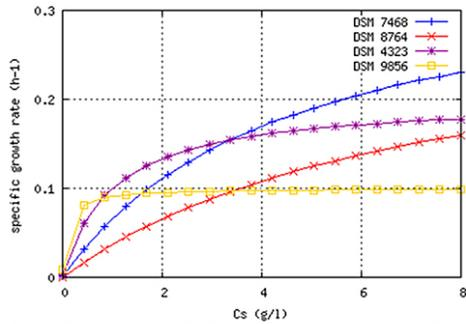
Several strains are added to **one** continuous reactor. The Monod kinetics for all the strains are well known, and are displayed above. The dilution rate is set at 0.1 h<sup>-1</sup>. Which of these strains will be in the reactor after a steady state has been reached?
