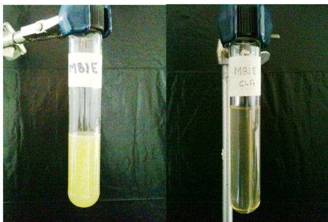
Fig. 2. Original M81-E sweet sorghum juice (left side as observed by reader) and clarified and centrifuged juice (right side).
